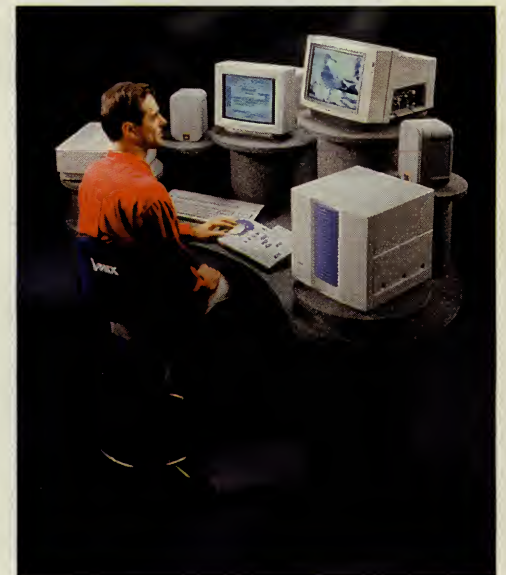
The ImMIX Video Cube is a complete on-line video-editing package that uses a Mac IIvx as its front end. It is the first Mac-based nonlinear editing system available that can record and play back video at 30 frames per second and 60 fields per second.
